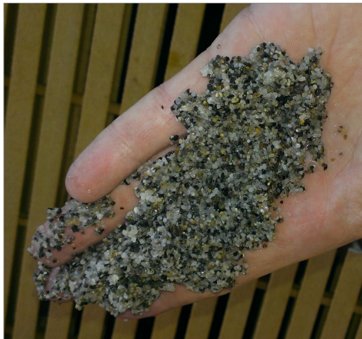
Sand Filter Media Entering the Grit King®
