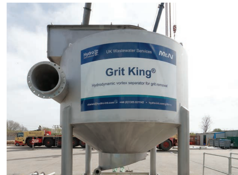
With no power requirement for separation and no moving parts the Grit King® has OPEX and is easy to maintain.
