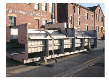
The Atlas Works installation under an urban road comprised two 700 x 2500 mm units with a maximum inlet flow of 1593 l/s (1 in 5 year) and a maximum screened flow of 1328 l/s (1 in 5 year).
